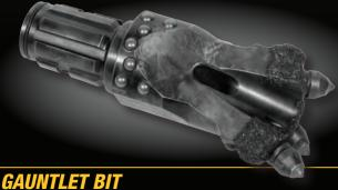
The Gauntlet bit was designed for use in soft to medium rock, shale and caliche ground conditions up to 10,000 psi (68.9 MPa) with exceptional steering capabilities. Carbide buttons are strategically placed on the bit for optimum cutting, while carbide hardfacing helps to enhance wear and performance characteristics. A replaceable three-tooth design delivers a consistent cutting structure for steering corrections to help maximize drilling performance.
